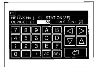
\*1 For the station, with either system specify "FF", which shows the PC CPU to be accessed, or "0" ~ "64".
